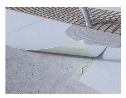
Note: DualProof C Membrane is designed for use with structural reinforced concrete. The concrete should be designed by a Structural Engineer to EN 1992. Please ensure that the concrete is placed and cured correctly, and that all non-movement construction joints are detailed with CEMflex Active Waterstop. Please consult our Technical Department for advice on the detailing Movement Joints and Non-Movement Joints.
