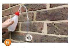
A Stormdry Gauge can be used to demonstrate the effectiveness of the treatment. The test should be carried out at least 28 days after applying Stormdry which allows the water absorption of the wall before and after treatment to be compared.
