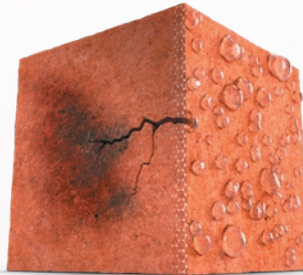
HAIRLINE CRACKS ARE UNPROTECTED, ALLOWING WATER INTO THE INTERIOR
